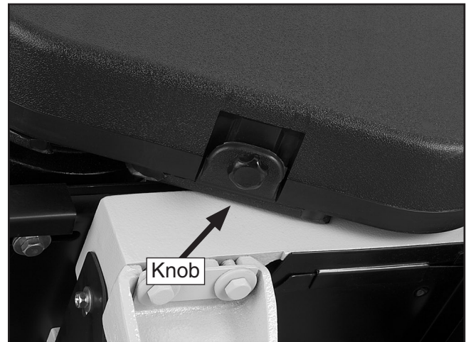
Figure 12 Secured pulley cover lid.
